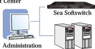
**Co-Hosted Solution** - the buzz word in telecommunications today is "hosted" solutions. One issue hosted solutions can not overcome is redundancy or latency of the last mile. The Sea Softswitch overcomes this obstacle by allowing a local processing engine to be located on the customer premise. The database for the customer is housed in the central NOC as well as on the customer premise. In case of a network failure the local Sea processing engine takes over and processes calls seamlessly.
